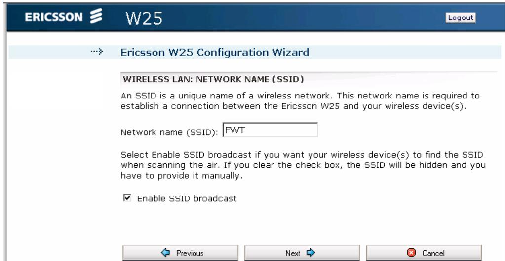
Figure 14 Wireless LAN: Network Name (SSID) page
