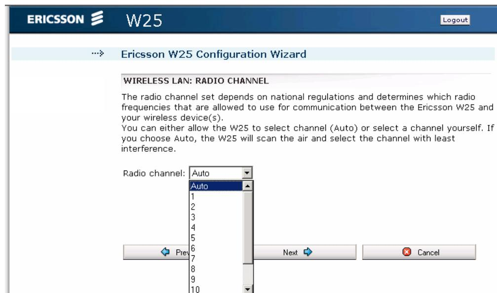
Figure 13 Wireless LAN: Radio Channel page
